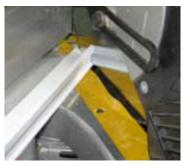
3. Notch back leg of nailfin to clear the weld.
