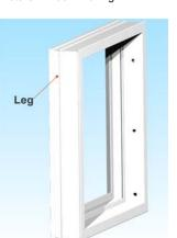
Mulling Side by Side 0204. Shown to the left is a picture window with leg. Remove the leg using router and edge quide.
