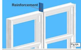
Cut the current excalibur reinforcement, the length is equal to window height minus 1/2". Note: the cut length is the same for any configuration. Insert reinforcement into the Mulled opening. Fig.
