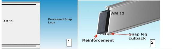
Process the snap legs on the AM 13 using the router. The cutback is 1/2 inch for 0404 and 1" for 0401. This will allow a clearance over the weld flash. Insert the reinforcement into AM 13(see fig 2). The reinforcement and mullion = window height
