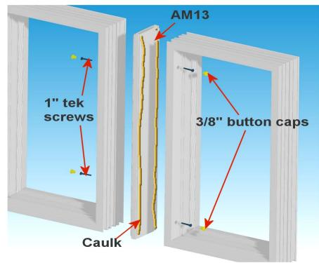
**Exploded view of the side by side Mull assembly for picture windows.** Counterbore through the **first wall of the extrusion** on the picture window 0404 (use a 3/8" counterbore with 5/32" pilot. Do this for both windows. Drill approximately 2" from either side of the picture window jambs
