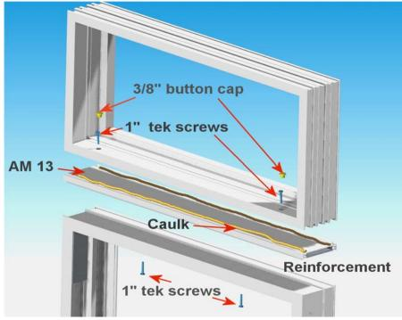
**Exploded view of the Stacked Mull assembly.** Counterbore through the **first wall of the extrusion** on the picture window ,0404 (use a 3/8" counterbore with 5/32" pilot. Do this for both windows. Drill approximately 2" from either side of the picture window jambs
