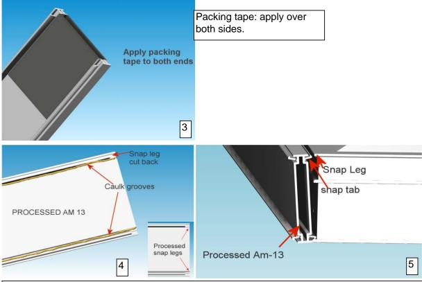
Caulk groove as shown. Attach the snap leg of the window frame to the snap tab on the AM13 mullion. Angle the Mullion on the bottom as shown. Attach the mullion snap tab to the snap leg of the frame on the bottom; using pressure snap the top half of the mullion together. Repeat this step for the opposite window.
