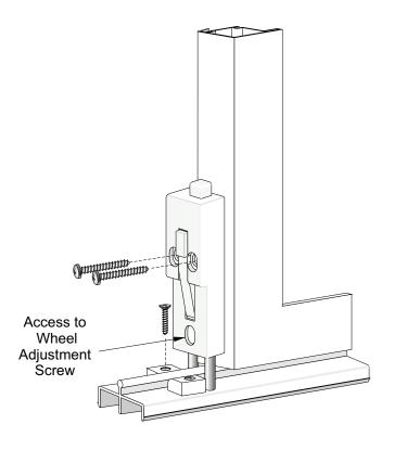
Locate lock pin stops last. Close and lock the panel. Place both lock pin stops as illustrated onto the track and secure with #8 x 1" flat head, phillips screws.
