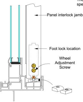
After the door is installed, make wheel adjustments if needed to align the panel with the strike jamb, to obtain an equal reveal, and adequate clearance between lock pin stops and panel.
